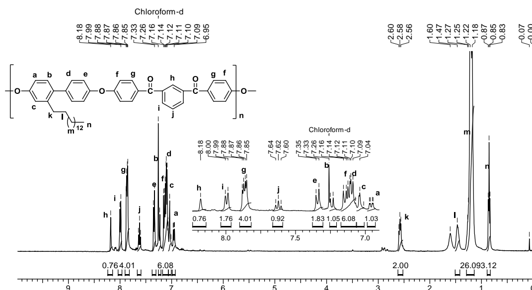
Figure 7.7 ^1\text{H} NMR spectrum (in \text{CDCl}_3 ) of poly(ether ether ketone ketone) (PEK-II) derived from PDBP and BFB
