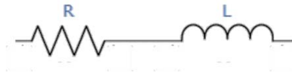
Figure 2B.18: Equivalent circuit for fitting the Nyquist plot, R represents the resistor and L inductor
