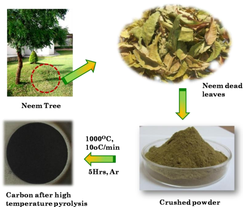
Figure 3.1: Schematic diagram for the synthesis of functional carbon from dead leaves and the supercapacitor based thereupon.
