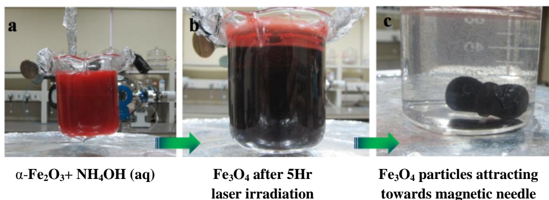
Figure 5.1: Conversion of bulk \alpha - \text{Fe}_2\text{O}_3 to \text{Fe}_3\text{O}_4 after 5Hr laser irradiation; a) \alpha - \text{Fe}_2\text{O}_3 in aqueous ammonia solution before laser irradiation; b) After 5 Hr laser irradiation showing formation of black colored \text{Fe}_3\text{O}_4 ; c) Magnetic \text{Fe}_3\text{O}_4 particles attracted to the magnetic needle after the stirring stopped
