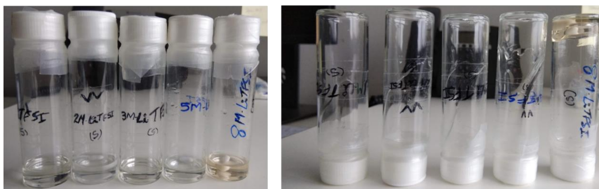
Figure 4.5. Digital images of the inversion tests of Li-P-X specimens showing the increment in viscosity with respect to an increase of LiTFSI content in PEGDME. (Reprinted (adapted) with permission from (ACS Appl. Mater. Interfaces 2020, 12, 1, 567-579). Copyright (2020) American Chemical Society).
