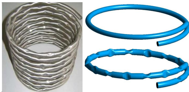
Figure 2.11 Geometry used in the model (A) simple helical coil geometry, (B) pinched tube helical coil geometry and (C) photograph of pinched helical coil tube
