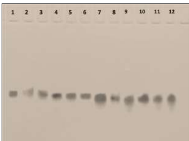
Figure 4: Denaturing gel electrophoresis of TBA, iso TBA oligomers, indicating their purity. Strand concentration of TBA and iso TBA sequences were 320 \mu M and gel was run in TBE buffer at 25 ^{\circ} C at 150V. The gel was visualized by UV- shadowing.
