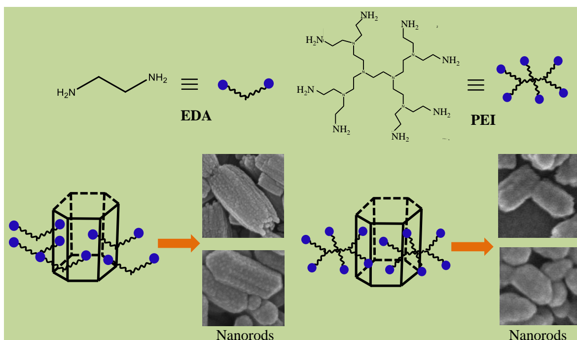
Scheme 2. The schematic representation shows the evolution of shapes of NaYF 4 : Gd 3+ , Tb 3+ phosphors using amine-functionalized ligands, EDA and PEI.
