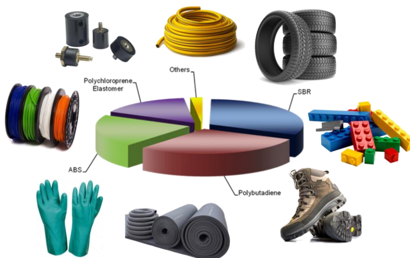
Fig. 1.4 BD as a precursor of synthetic rubber
