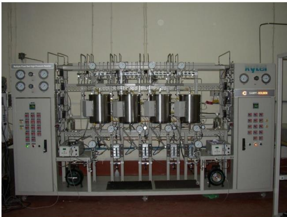
Fig. 2.9 Fixed bed reactor system used for testing catalyst.
