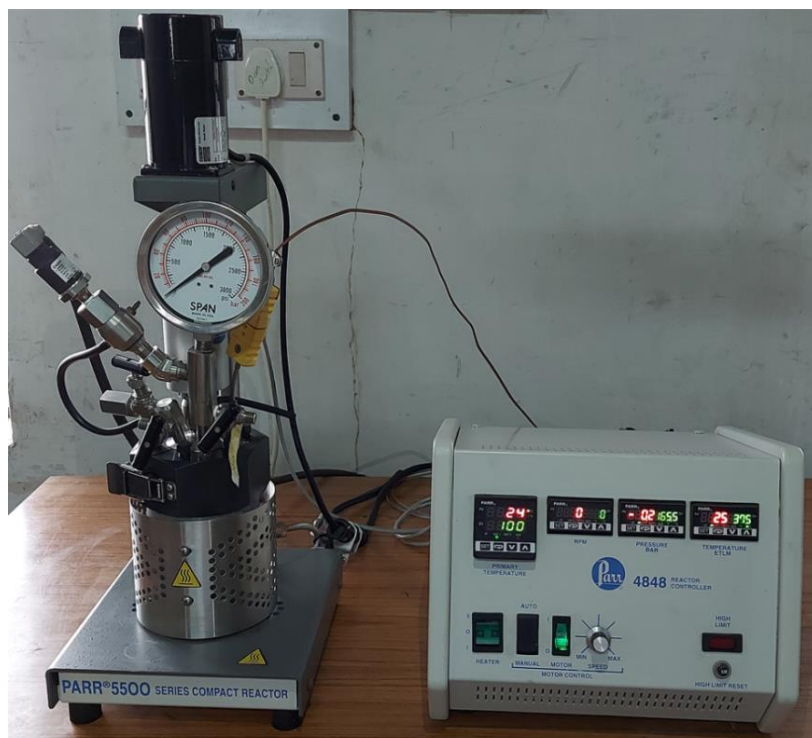
Fig. 2.10 Parr reactor setup.
