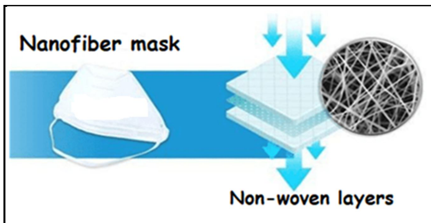
Figure 1.3: Biomaterial based non-woven nanofiber face masks. Adapted from website of Azonano, Image credit: Inovenso. 13
