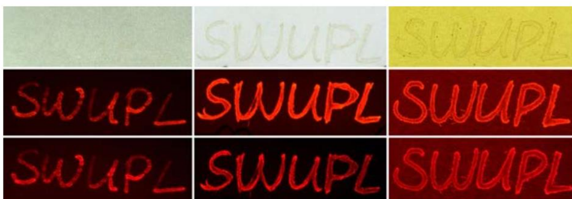
Figure.16. Anti-counterfeit ink images of handwriting on several types of paper using as-prepared fluorescent Au NCs. Weighing paper, regular office paper, and Kraft paper, from left to right. Adapted from Ref.69. 69
