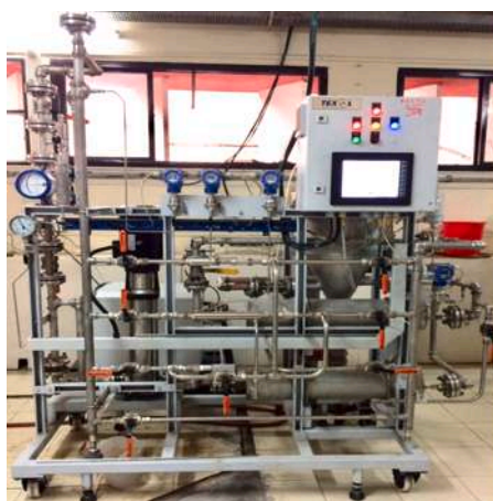
Fig. 2. Schematic of hydrodynamic cavitation pilot plant and experimental setup
