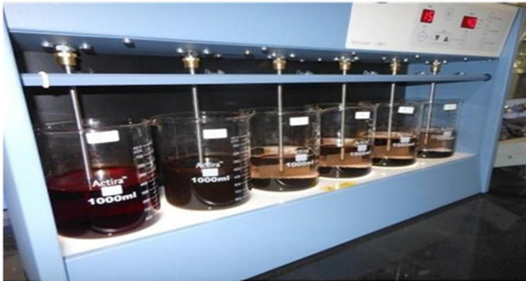
Figure 2. 3: Jar test apparatus for coagulation experiments [1]
