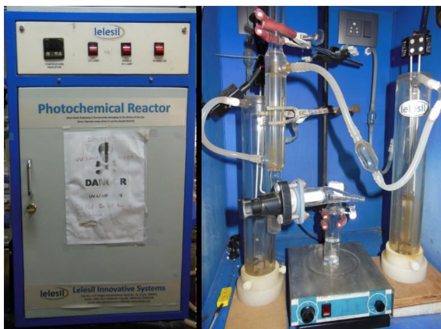
Fig.2.4. The photographic image of the photochemical reactor
