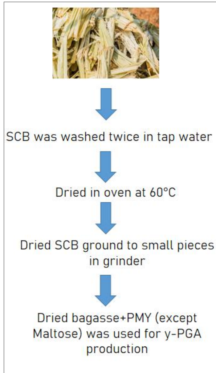
Fig. 5.20. Schematic of Poly-gamma-glutamic acid production from sugarcane bagasse
