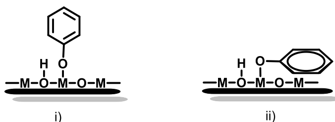
Scheme 4.4. Adsorption of phenol onto catalyst i) perpendicular orientation and ii) parallel orientation
