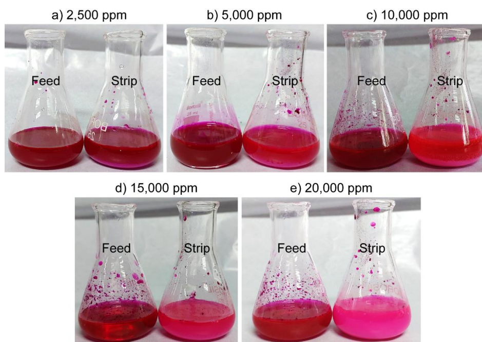
Fig. 5.4. Feed and strip side of ammonia titrated with barium chloride after transport study.
