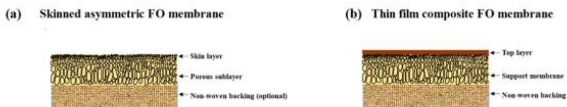
Fig. 1.13. Illustration of the structure disparity of (a) skinned asymmetric membrane and (b) TFC membrane [1] “Reprinted from Membranes, 12, Tian, et al., Forward osmosis membranes: the significant roles of selective layer, 955-976, Copyright (2022), Licensee MDPI, Basel, Switzerland”.
